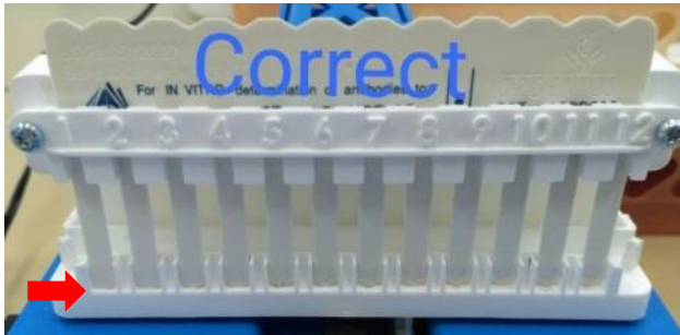
Fig.9 Correct Comb placement Comb is gently pushed down at both sides until reaches stop
